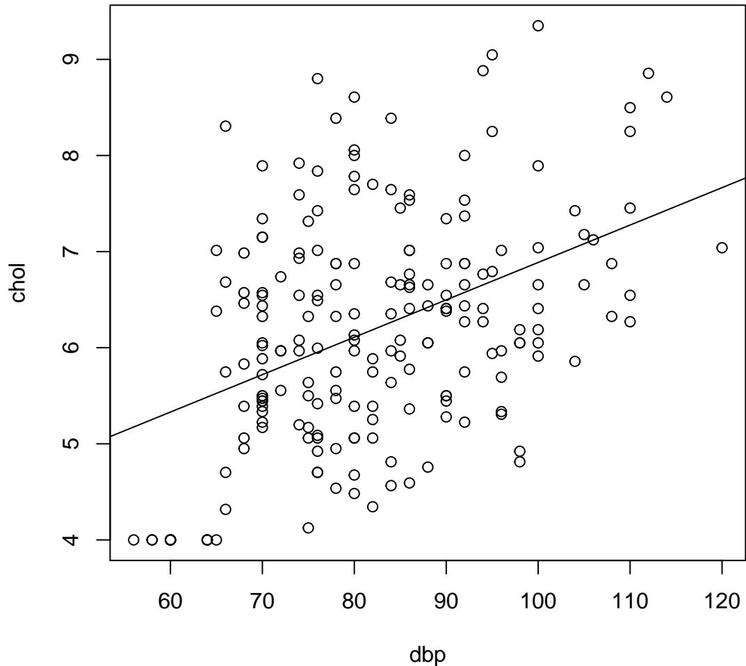
this allows assessment of normality, linearity and equal variance assumptions. We expect eliptical/oval shape (normality), equal scatter of dots on both sides of the prediction line (equal variance). Both these indicate linear relationship between chol and dbp.
