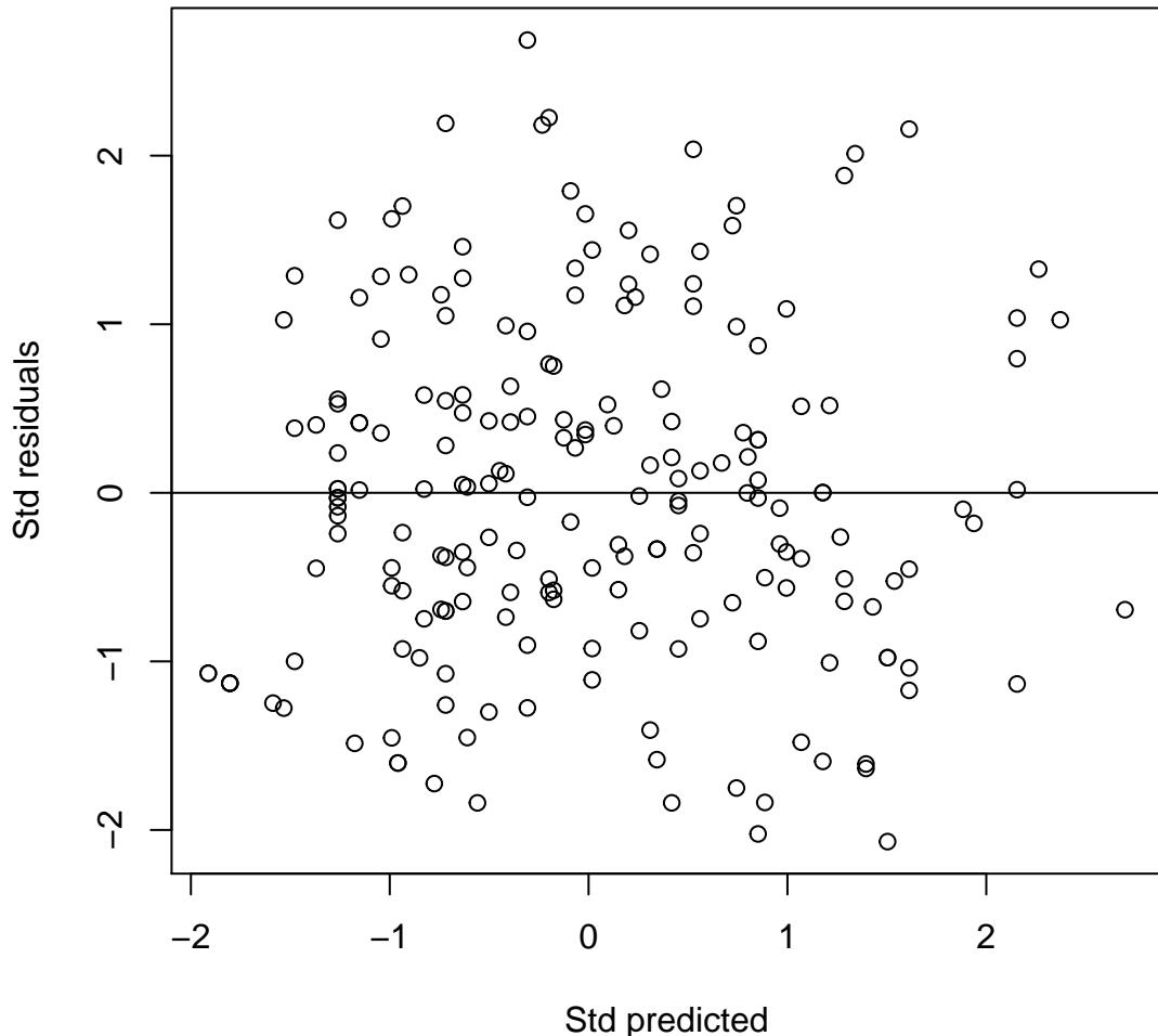
The dots should form elliptical/oval shape (normality) and scattered roughly equal above and below the zero line (equal variance). Both these indicate linearity.
